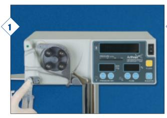
Following removal of the orange cap, the pressure sensor line is plugged into a snap-fit connection located on the lower left corner of the front panel.
